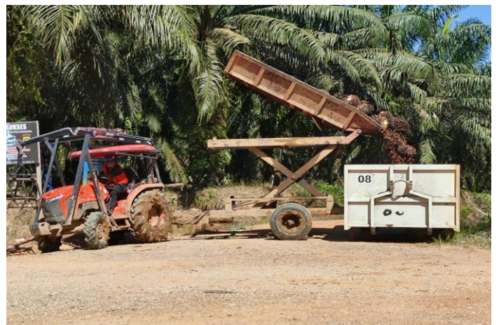
Figure 8. Palm Crane with Scissor Dump System
