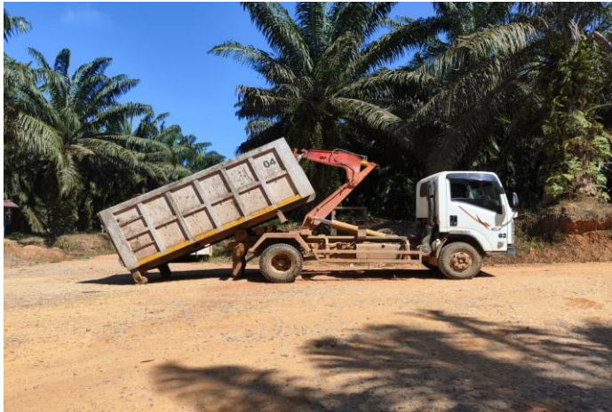
Figure 9. Lifting the Container
